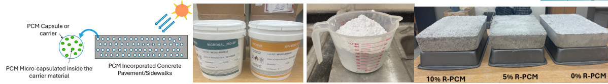
Figure 1: Research Methodology; PCM Powder Form; Three Conc-PCM slabs
